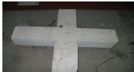
Fig.13 Model of intersecting beams before test
